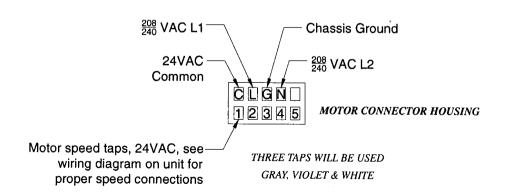
Caution: High efficiency brushless DC motors are wired with power applied at all times (G.E. X13 for example), see illustration above. Low voltage thermostat demand and board algorithms will control its use.
